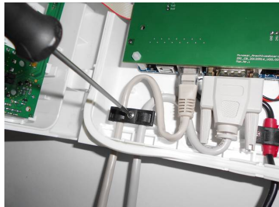
Image 5: Connect the network cable, mount the strain relief
