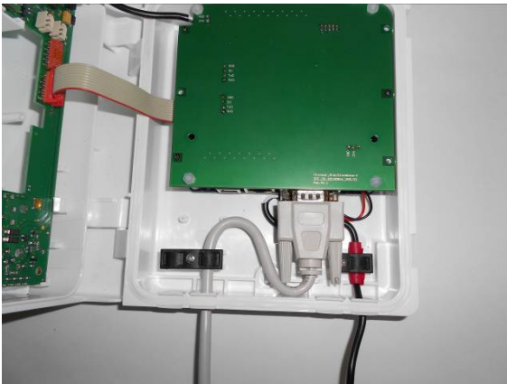
Image 2: Open the CommunicationMaster housing
