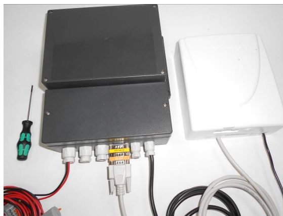
Image 1: Connect the CommunicationMaster to a level converter using the attached Gender Changer.
